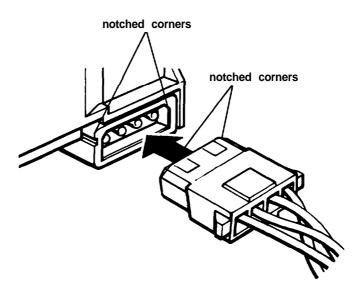
Make sure the holes fit over all the pins and then push in the connector.
